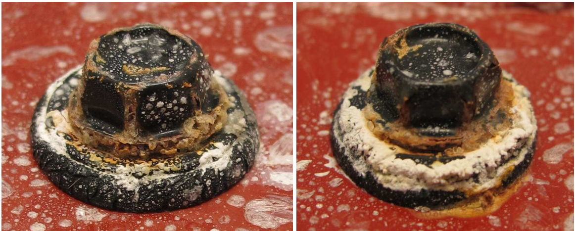
Figure 4. Screws A (Würth) ja E (Berner) after 425 hours test time.
