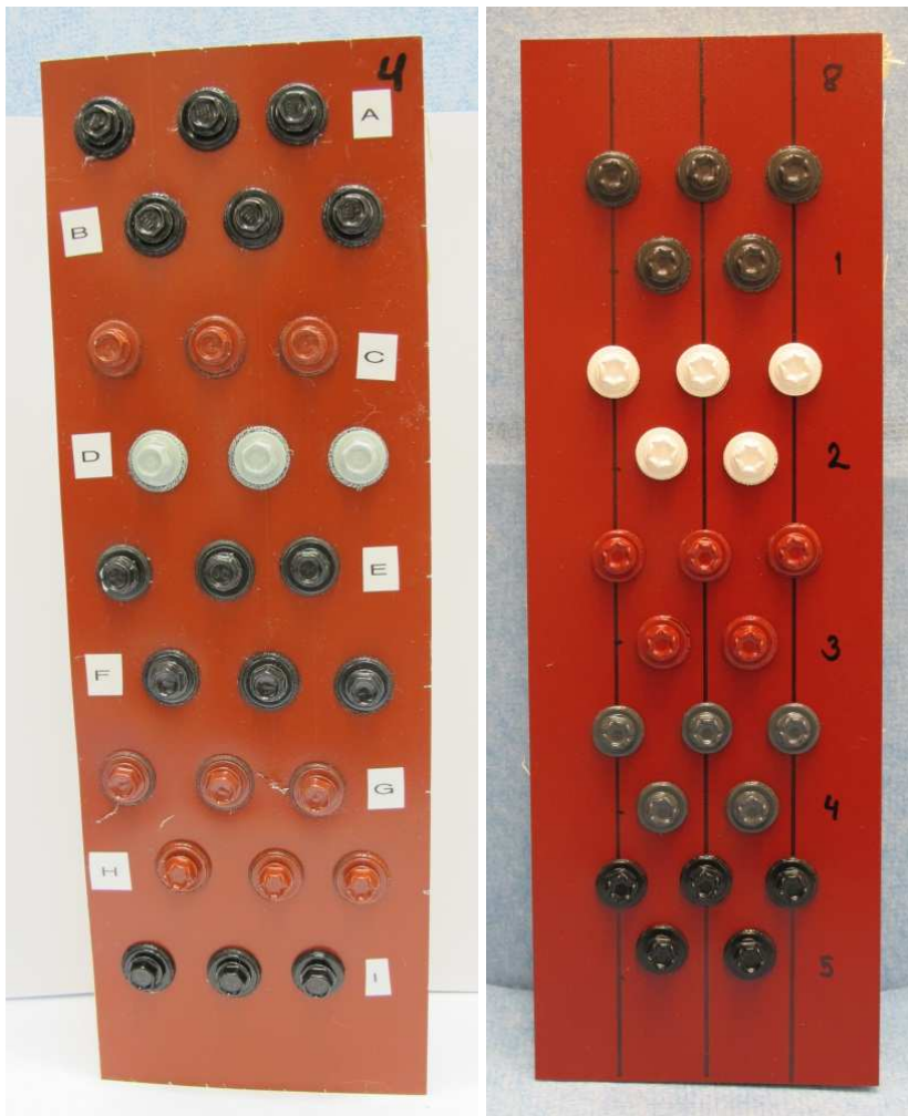
Figure 3. Screws mounted on the sample racks before the test. Left rack contains the screws of other manufacturers and the Kingi screw with top coat only. The right rack contains the Kingi screws randomly taken from the manufacturing and from the stock.
