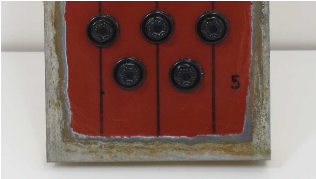
Figure 6. Kingi screws and Pural thin sheet after test. Delaminated paint is removed.
